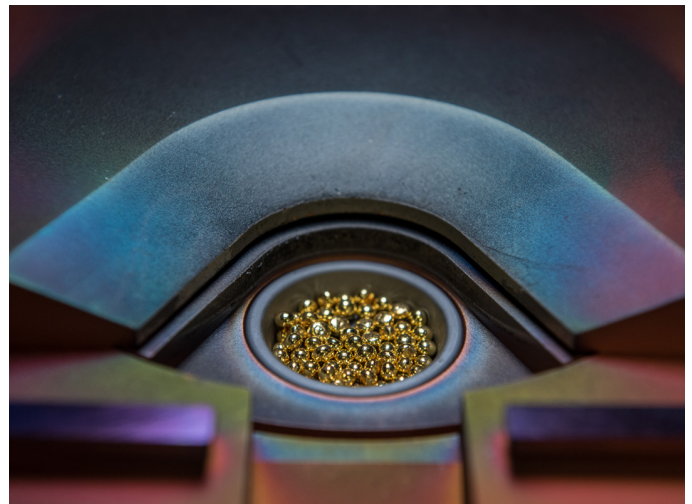
A gold-filled crucible within an electron beam source demonstrating an appropriate 80% fill level.
