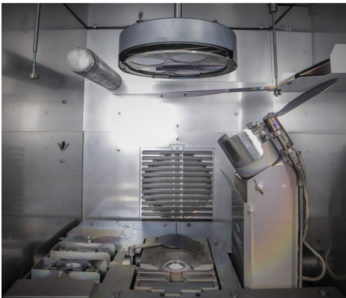
An electron beam evaporation system demonstrating a long source-to-substrate distance, appropriate for temperature sensitive substrate materials.
