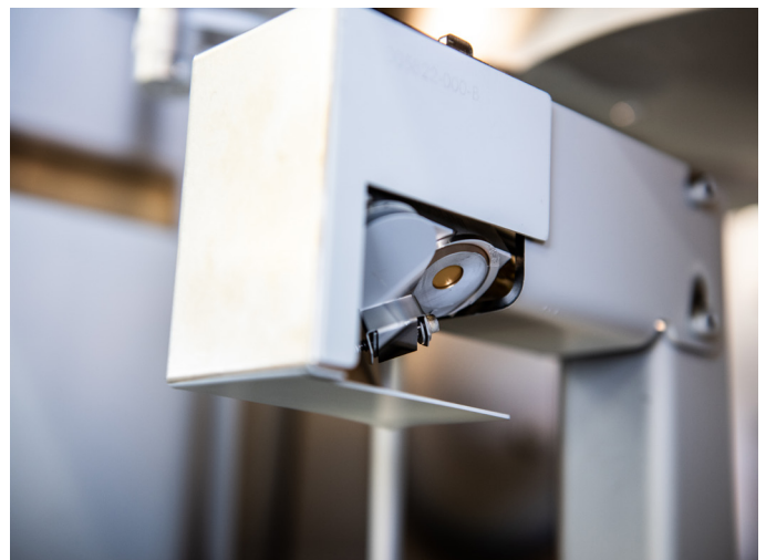
A dual quartz crystal microbalance often used for measuring instantaneous rate and thickness of electron beam deposited films.
